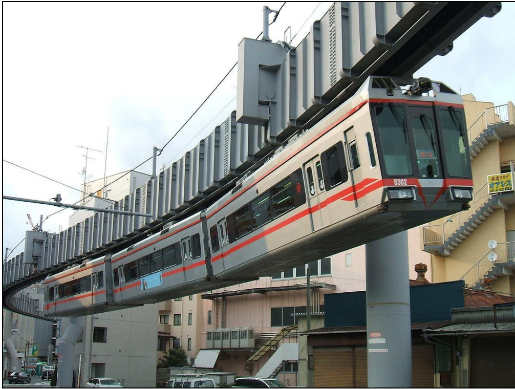
2010's-61: Three-car "suspended monorail" operated by Shōnan Monorail between Enoshima and Ōfuna (orange stripes having been replaced by black stripes by 2019) (2008/08/10) [ en.wikipedia.org/wiki/Shonan_Monorail ].
