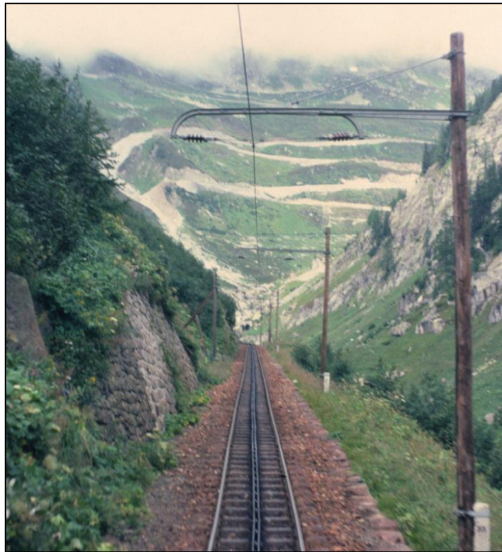
1970's-27: Looking back and down from the last car of Furka-Oberalp's Glacier Express , the rack evident on this stretch west of Andermatt (1978/09/07) [PETER DAWES].
