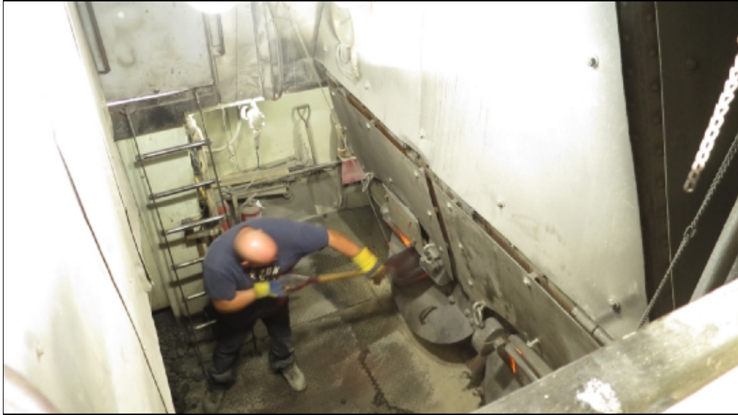
2010's-63: Stoker feeding the furnace of Muskoka Steamships' coal-fired SEGWUN, during evening dinner cruise (2018/07/21) [SANDRA DAWES].
