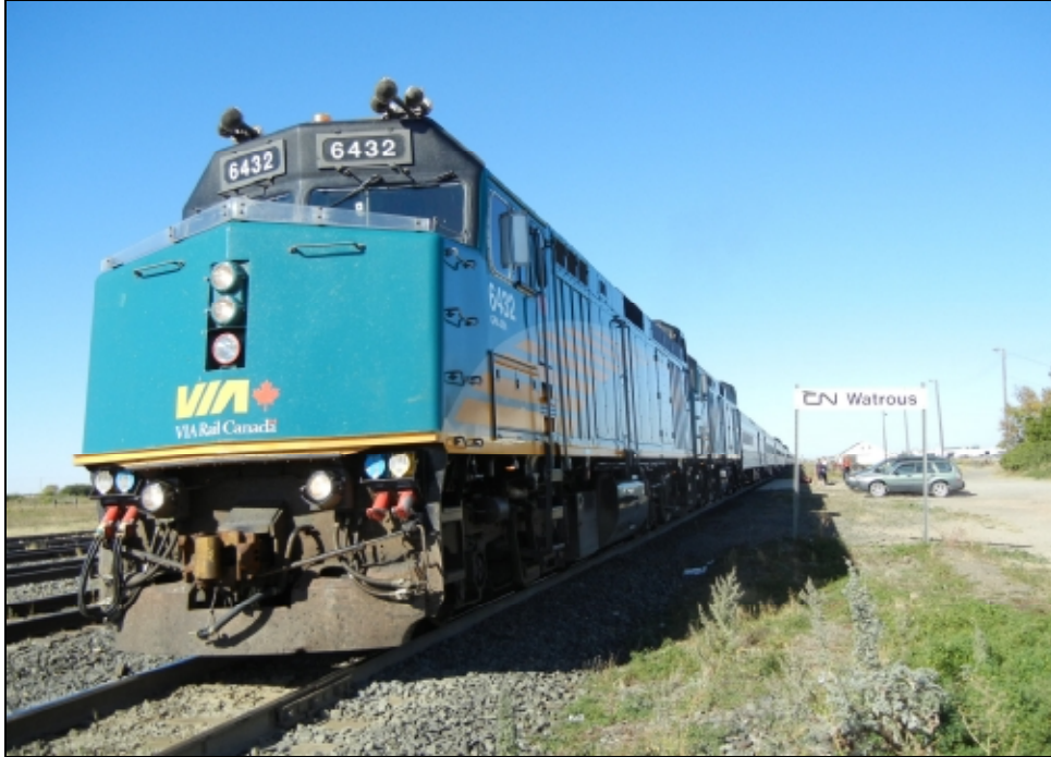
2010's-22: VIA No. 2 Canadian , newly arrived at Watrous SK from Vancouver and Edmonton, on its way to Toronto, led by two rebuilt F40PH-2's (2013/09/24) [SANDRA DAWES].
